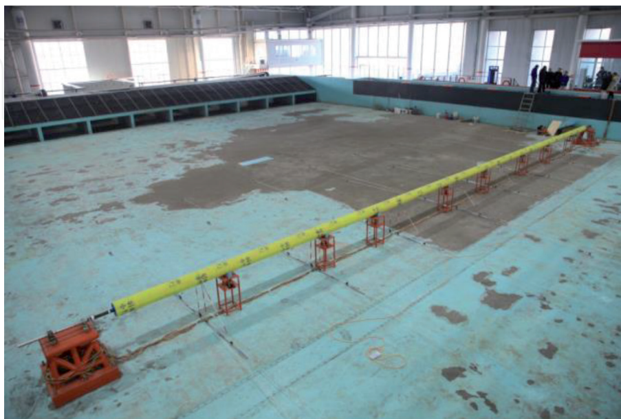
Figure 17. Photo of SFT overall structural behaviour test sponsored, designed, and led by CCCC; SFT model and sensors prepared by DUT; and basin built by TIWTE.
