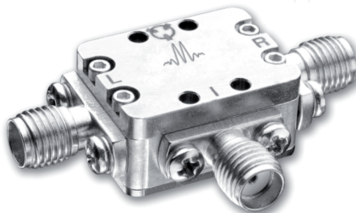
Figure 11. Example of connectorized mixer (photo courtesy of Marki Microwave).
