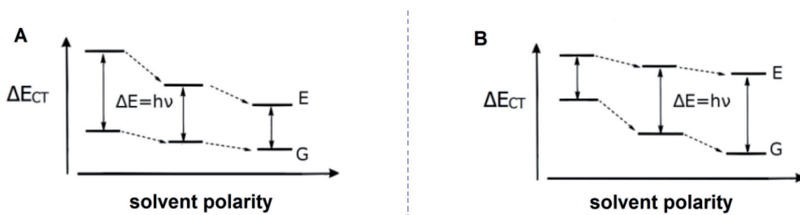
Figure 9. Plots of CT energy as a function of solvent polarity corresponding to (A) positive and (B) negative solvatochromism (G corresponds to ground and E to excited state).
