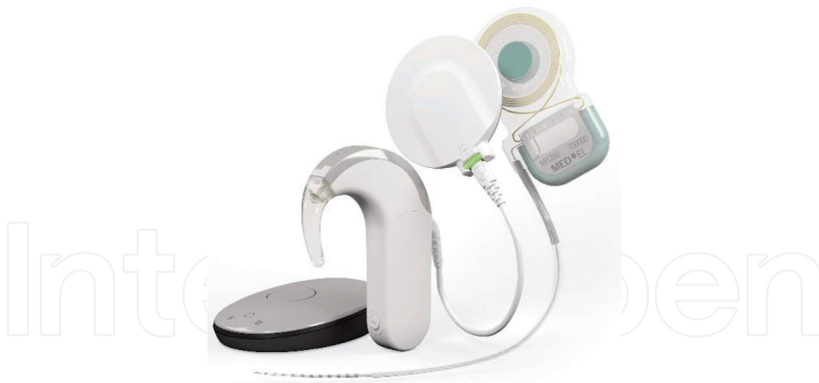
Figure 4. Image of a cochlear implant showing the implanted and externally worn audio processor parts (behind-the-ear audio processor and single unit audio processor (courtesy of MED-EL GmbH).
