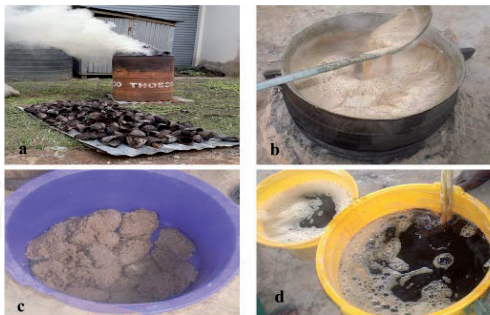
Figure 7. Stages in local soap production from agricultural waste. (a)–(d) represent ashing of dried cocoa pods/plantain waste in a carefully constructed metal drum, the soap production process, finished product in solid form and finished product in liquid form, respectively.
