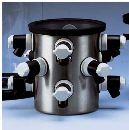
Figure 3.2. The freeze dryer system (Labconco, USA) used for lyophilization of chitosan-based membranes.
