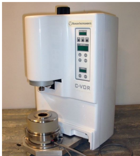
Figure 3.3. The C-VOR rheometer (Bohlin Instruments, USA) used in this study.
