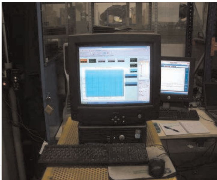
Figure 3. Data acquisition system for the compression test.
