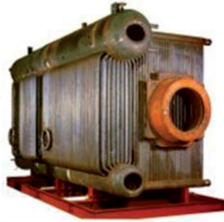
Figure 5. Typical water-tube steam boiler.
