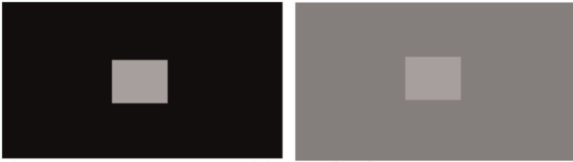
Figure 8. Simultaneous contrast phenomenon perceived at the different dark backgrounds in luminance values.
