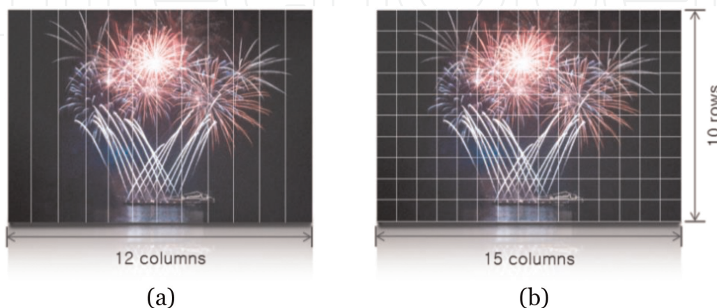
Figure 2. LCD TVs according to local dimming method. (a) LCD TV with edge-lit backlight. (b) LCD TV with direct-lit backlight.
