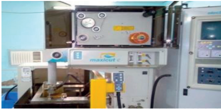
Figure 1. D2 steel machining using WEDM process.
