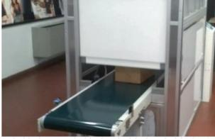
**Figure 3.** *RFId reading post, Box label printing and application. Source: Oscalito.*
