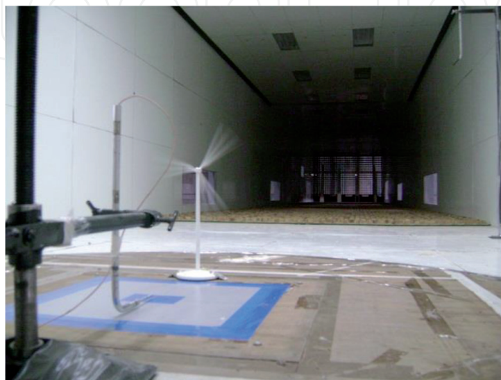
Figure 20. Wind turbine model spinning during the wind tunnel test.
