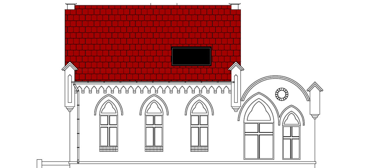
Figure 4.84 Location of solar panel on roof slope.
