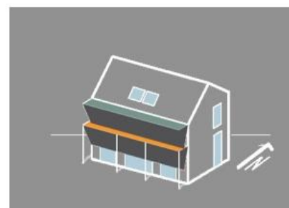
Figure 2.4 Shading elements on the south facade
