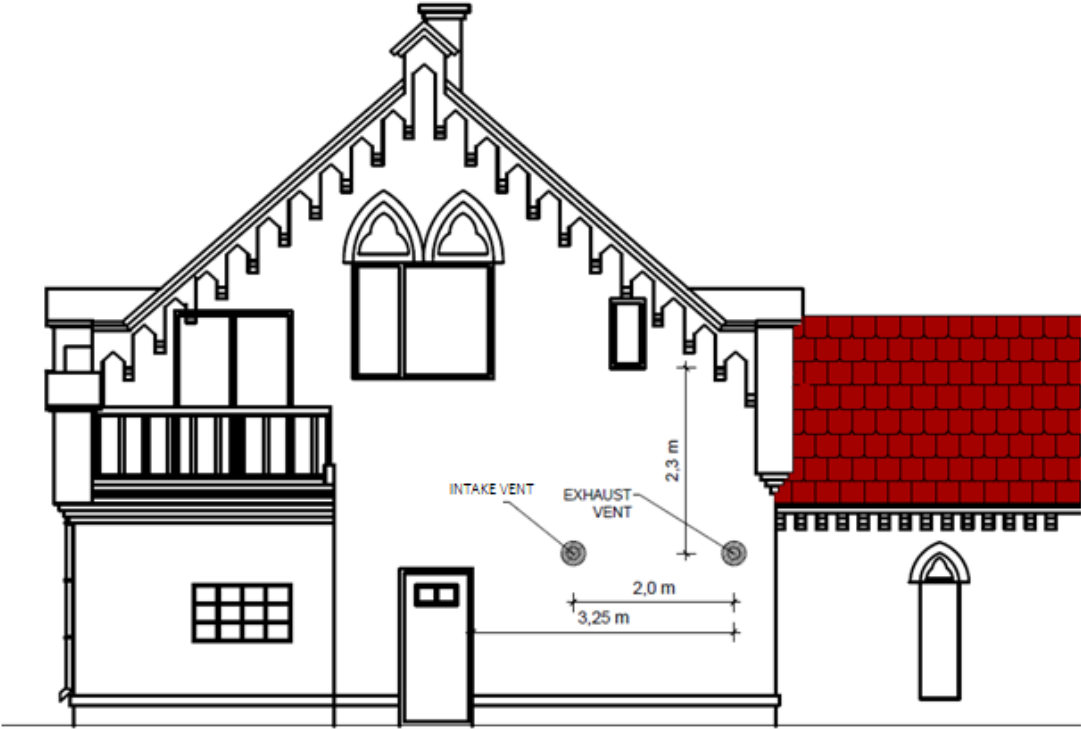
Figure 4.75 Part of the eastern elevation of the building – location of exhaust and inlet vent.
