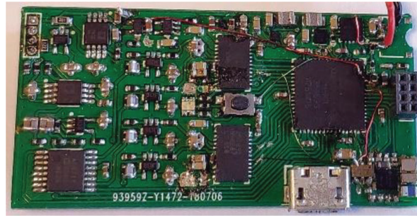
Figure 4. Image of the 32-bit impedance acquisition system prototype.
