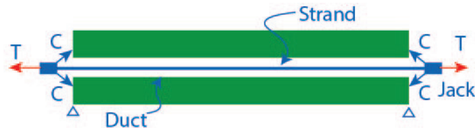
Figure 2. A simplified illustration of the mechanism of prestressing.
