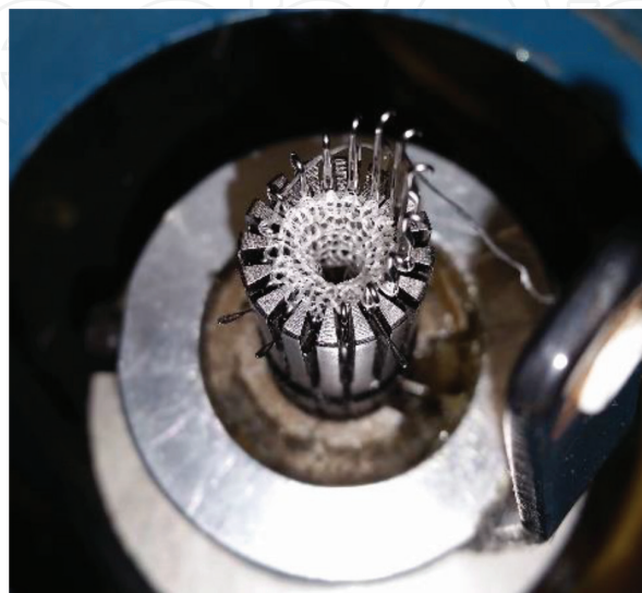
Figure 12. The circular knitting machine for weft knitting tubular fabric.
