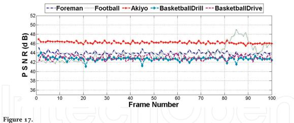
PSNRs of the proposed watermarking method when HEVC process is applied.
