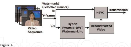
The block diagram of the watermarking process with the application of HEVC process.
