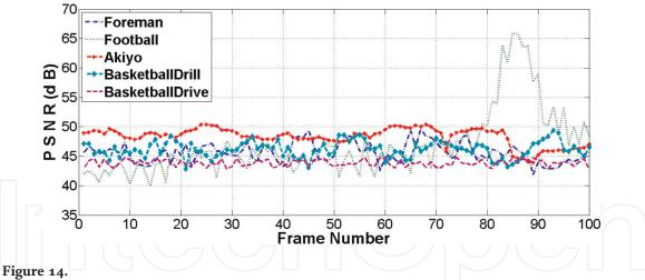
PSNRs of the test videos when the proposed watermarking process is used.
