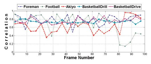
**Figure 18.** Normalized correlations of the proposed watermarking method when HEVC process is applied.
