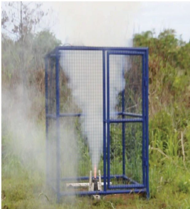
Figure 7. Static test rigs with single motor.
