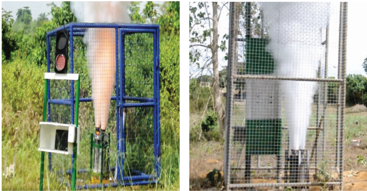
Figure 8. Static test rigs with tri-cluster rocket motors.
