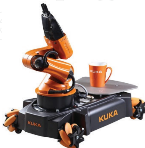
Figure 7. KUKA's youBot mobile manipulator (image courtesy: http://www.youbot-store.com/ ).
