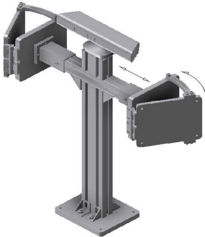
Figure 3.3: 3D model of a solution to the structure that allows to adjust the angle and the distance between the two arms assembled in sideways of the torso.
