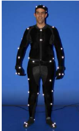
Figure 2.8: Example of optical system used for motion capture (Dinis, 2011).
