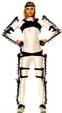
Figure 2.6: Application example of mechanical motion capture system (Metamotion, 2012).
