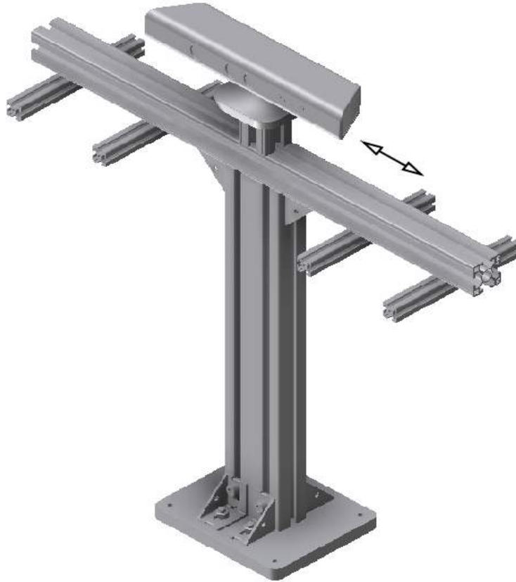
Figure 3.4: 3D model of a solution to the structure that allows to adjust the distance between the two arms assembled vertically to the torso.
