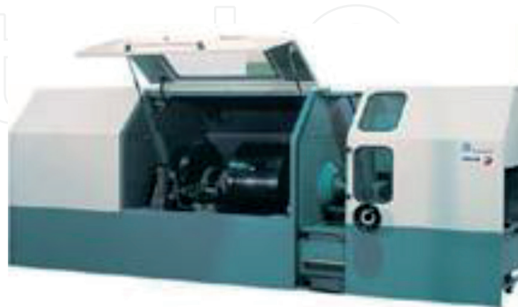
Figure 9. Disc brake testing machine, designed and constructed by TEKNIKER for Fagor Ederlan company.
