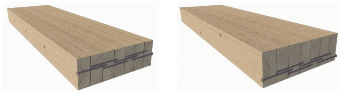
Figure 9. NLT with linear (left) and staggered (right) nailing patterns.
