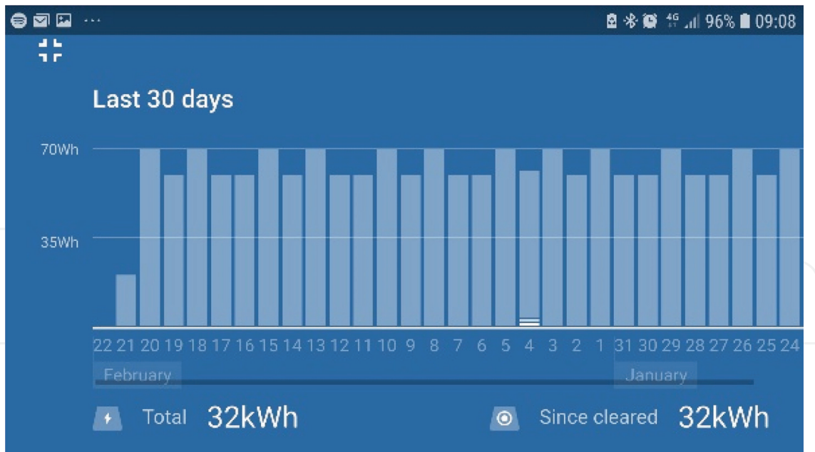
Figure 6. January 24 to February 21, 2019 3G system power consumption. The February 21 reading is less due to the time of day the readings were taken.
