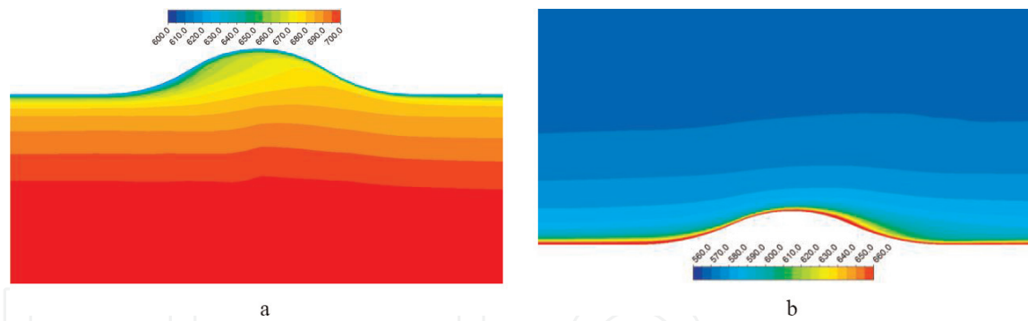
Figure 10. Temperature distribution at tube side and at shell side. (a) tube side; (b) shell side.
