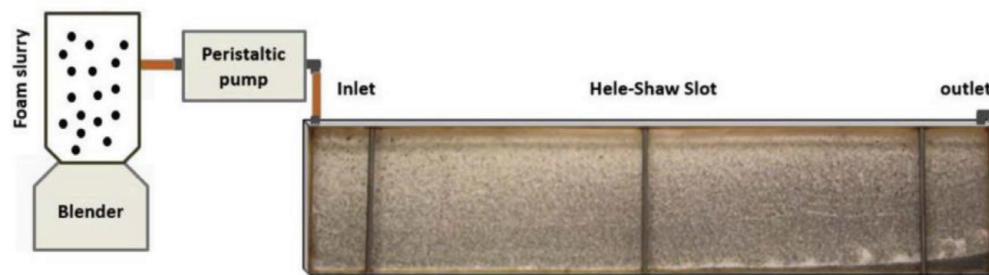
Figure 8. Laboratory scale Hele-Shaw fracture slot for mimicking induced fracture [98].
