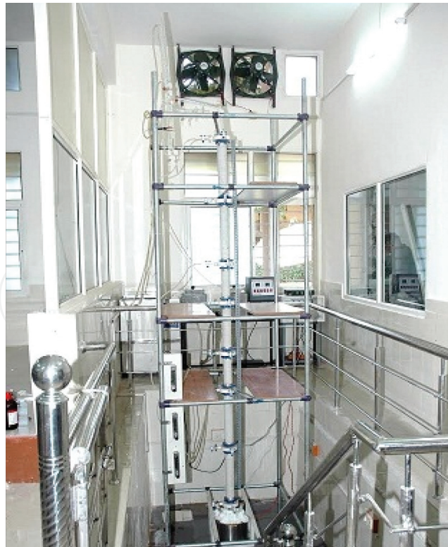
Figure 4. Pilot-scale reactive distillation column.
