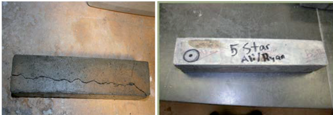
Figure 10. Significant number of freeze-thaw cycles.
