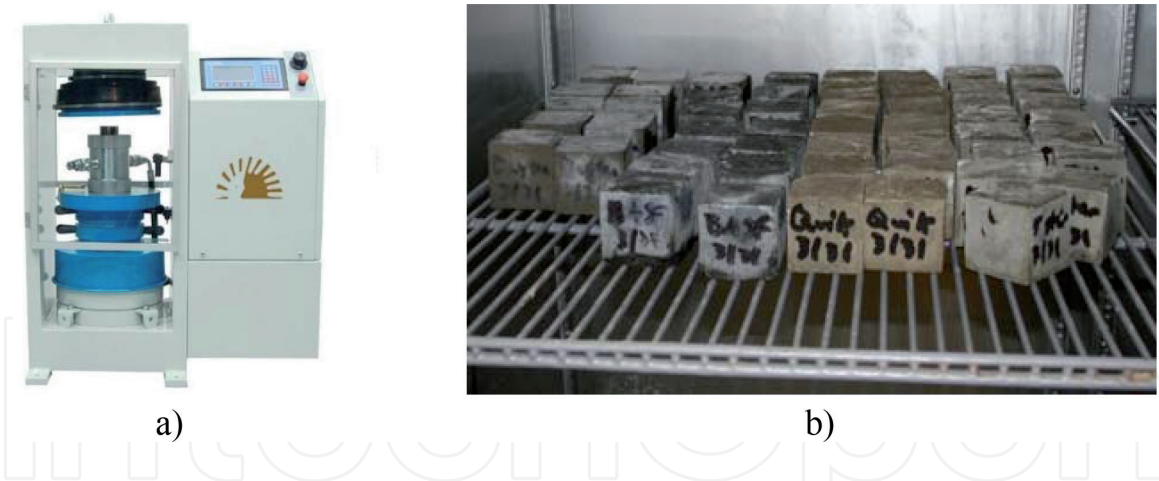
Figure 3. (a) Compressive test machinery. (b) Cube concrete samples.
