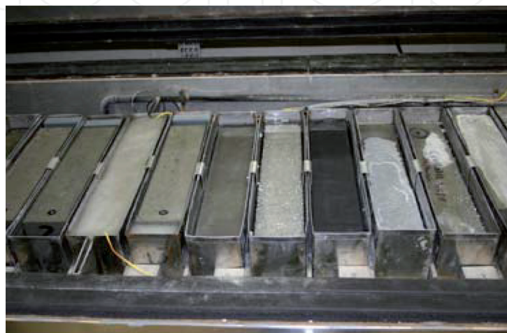
Figure 9. Durability investigation of the concrete, and freeze-thaw test.
