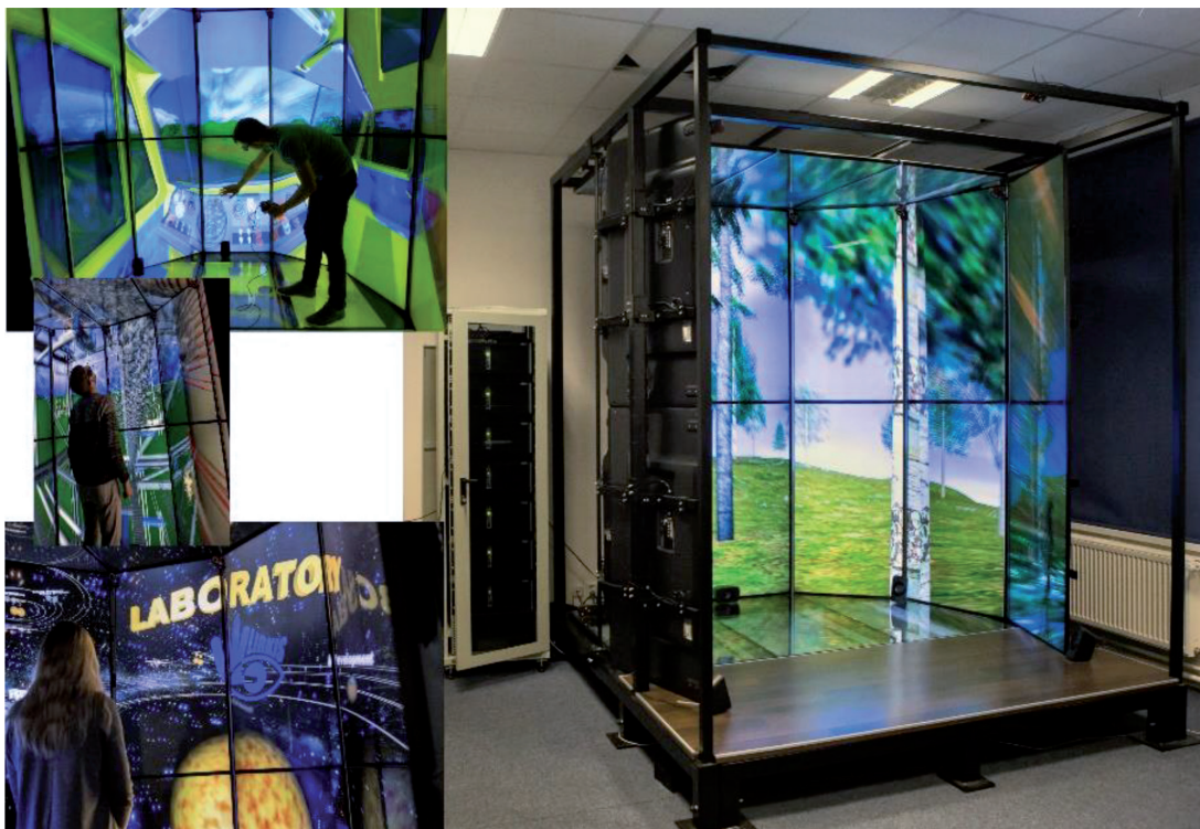
Figure 1. Virtual cave in laboratory LIRKIS at technical University of Košice and the examples of immersive visualization in this environment.
