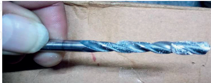
Figure 9. Adhesion of material to the drill bit.
