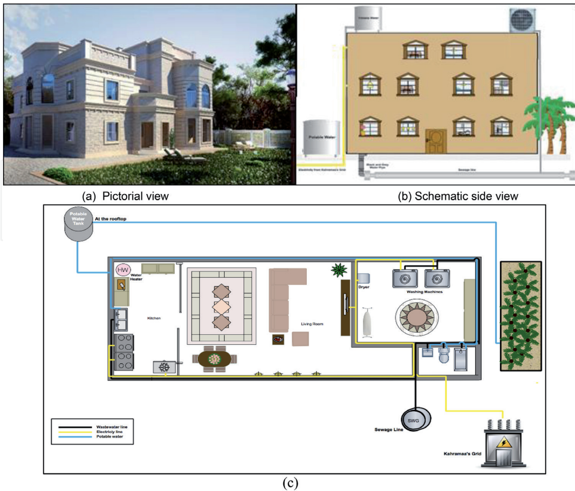
Figure 1. Case study villa: (a) pictorial view; (b) schematic side view; and (c) schematic plan view of the main water and electricity consumption points in a typical villa.
