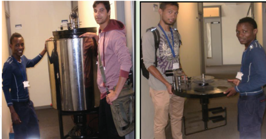
Figure 9. A home cottage industry ‘Two speed’ fluids mixer—as designed by MED students left—the assembled unit. Right—the counter-rotating slow speed mechanism (Watch online video at: https://www.youtube.com/watch?v=VymLqK9DDeo ).
