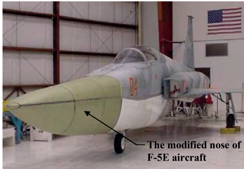
Figure 3. The F-5E aircraft modified by Northrop Grumman [23].
