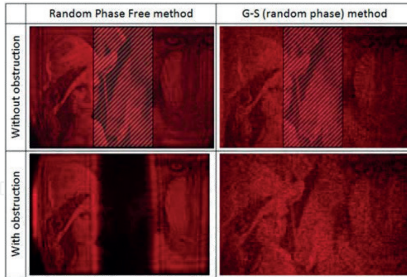
Figure 12. Resistance to large obstruction of the SLM visible in experimental projections from CGHs calculated with RPF method and G-S method [10].
