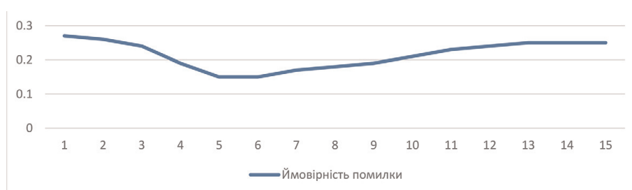
Figure 3. Error probability for different rules number in FNN.
