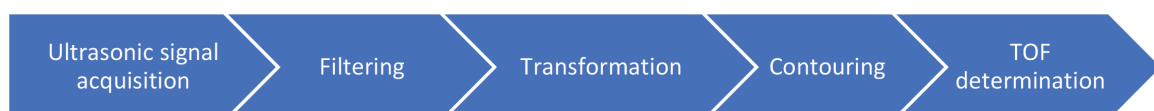
Figure 2. The sequence flow chart of the signal processing procedure for the analysis.
