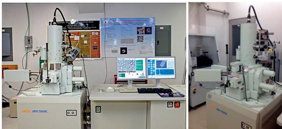
Figure 6. Two views of the JEOL JSM-7600F scanning electron microscope (SEM) setup.
