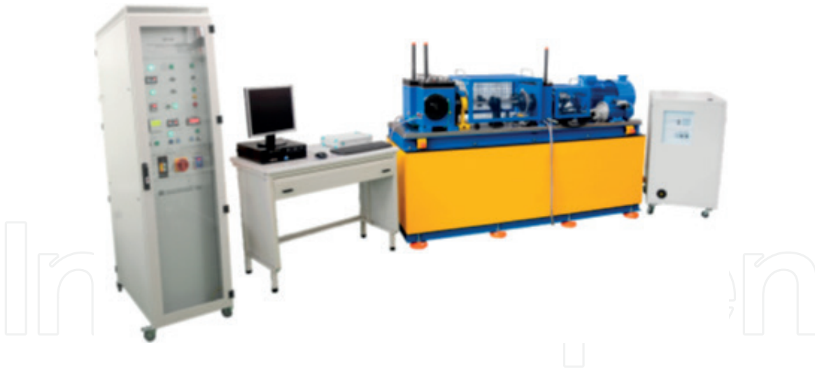
Figure 8. Photograph of the T-30 back-to-back bevel gear test rig with its control and measuring system (on the left) and water circulating cooling system (on the right) [44].
