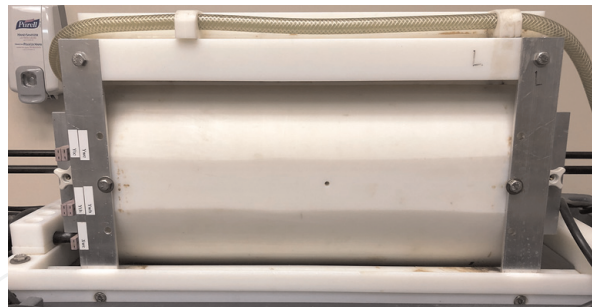
Figure 8. High performance water cooled insertable gradient set with maximum gradient at 50 G/cm, 17 cm in diameter and slew rate = 2100 mT/m/s used for high-resolution ^3\text{He} imaging.
