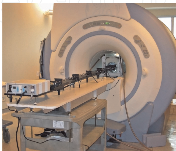
Figure 7. GE 3 T clinical MRI scanner using an external gradient set for rodents and the integrated custom-built flexiVent ventilator for mice.
