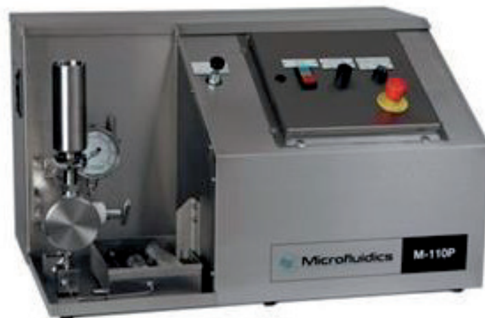
Figure 1. Typical high pressure homogenizer equipment.
