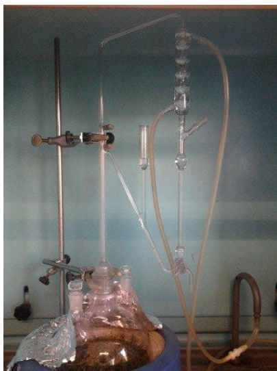
Figure 15 The Clevenger-type apparatus used in this work for the extraction and quantification of essential oils.
