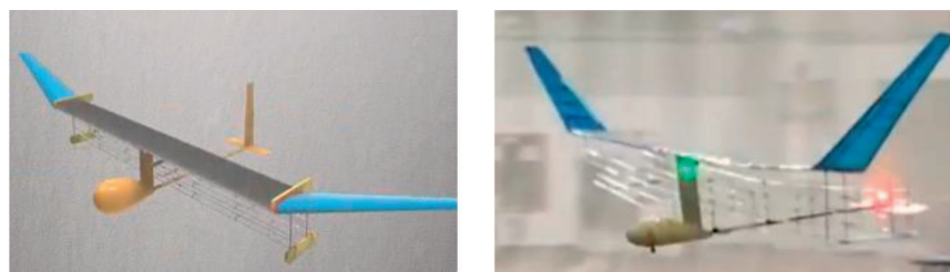
Figure 2. The first no moving parts aircraft by using the electrostatic energy [17].
