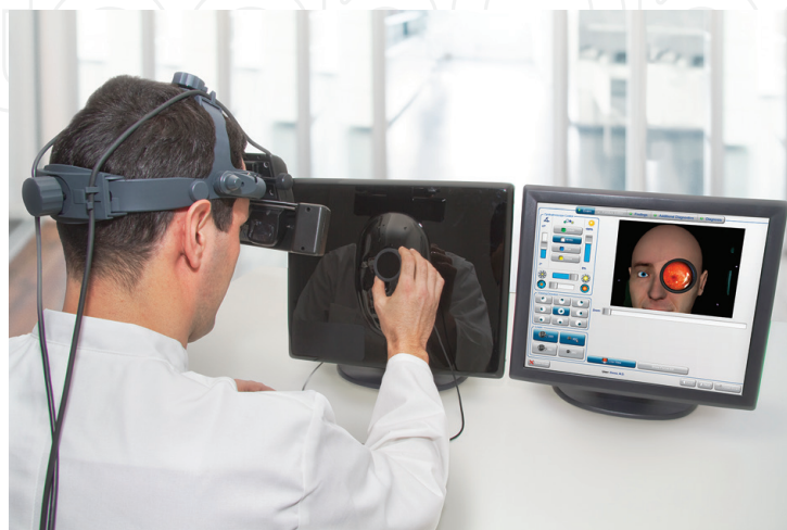
Figure 11. The VRmagic indirect ophthalmoscope allows users to develop the skillset for binocular indirect ophthalmoscopy with a 20D and 28D lens and records the percentage of the retina visualized in focus by the examiner.
