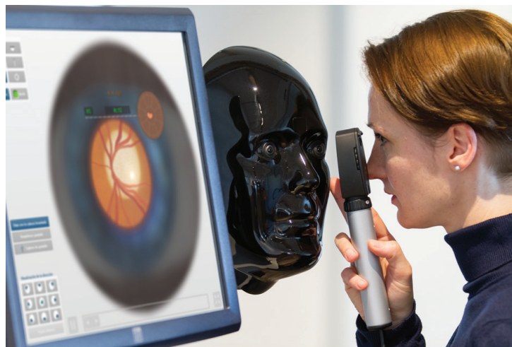
Figure 10. The VRmagic direct ophthalmoscope allows users to develop the skillset for direct ophthalmoscopy by progressively moving through skill modules and case pathology.
