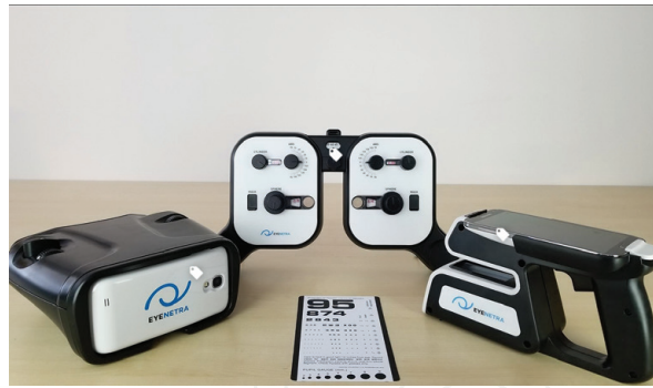
Figure 3. The EyeNetra system includes an autorefractor, lensometer, and a phoropter (shown adjacent to a standard near card for size comparison).
