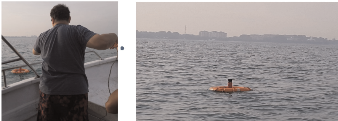
Figure 1. Deployment of Aquadopp 2 MHz current meter in the coastal water.
