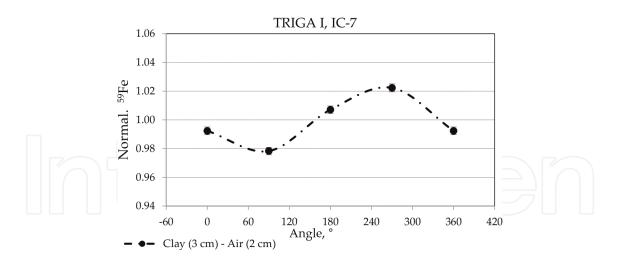
**Figure 5.** Radial gradient for thermal neutrons in clay-air in the IC-7 irradiation channel of the TRIGA reactor. The values are normalised related to <sup>59</sup>Fe and error bars are calculated based on the average statistics counting of 1099.3 and 1291.6 keV from <sup>59</sup>Fe, Vial 4 [37].
