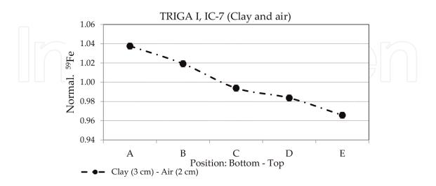
**Figure 4.** Axial gradient for thermal neutrons in clay-air in the IC-7 irradiation channel of the TRIGA reactor. The values are normalised related to <sup>59</sup>Fe and error bars are calculated based on the average statistics counting of 1099.3 and 1291.6 keV from <sup>59</sup>Fe, Vial 4 [37].
