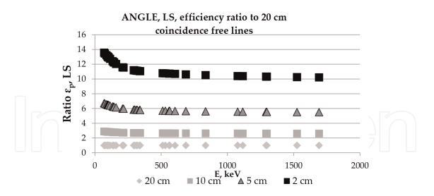
Figure 3. Gamma efficiency normalised to 20 cm obtained by ANGLE software for the large cylindrical sample, LS, Vial 1.
