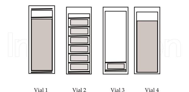
**Figure 1.** Vials prepared to carry out the experiments: Vial 1, large sample with reference material; Vial 2, with six small samples with reference material; Vial 3, with one small sample filled with reference material and Vial 4, with large sample filled with soil.
