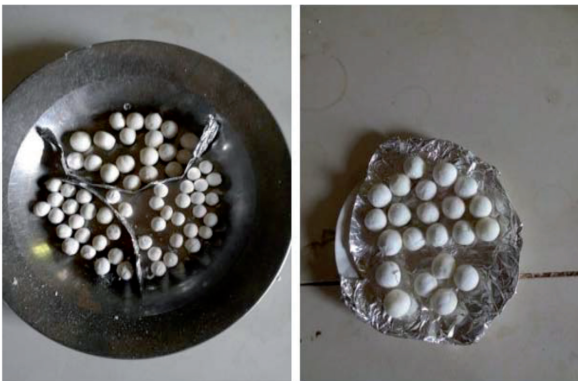
Figure 8. Coated urea of various coating thickness.
