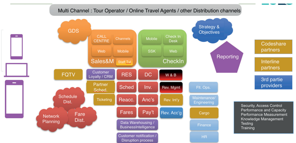
Figure 3. Typical airline IT architecture. Abbreviations used: GDS global distribution system, FQTV fare quote system, schedule distribution, fare distribution, RES reservations, Sched scheduling, Reacc. Reaccommodation, Inv. inventory, Anc's ancillary services, Pay't payment, W&B Weight and balance, Rev.Mgmt. Revenue management, RevInt'y revenue integrity, Rev. Acc'g revenue accounting, Flt ops flight operations, HR human resources, API application programming Interface, AI artificial intelligence, ML machine learning, IOT internet of things, AR/VR stand for augmented reality and virtual reality.
