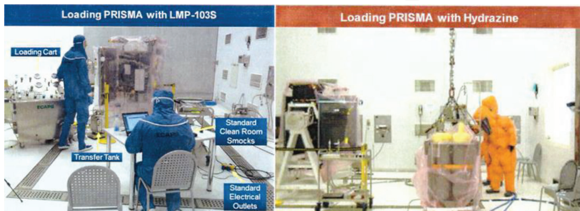
Figure 8. Propellant loading of satellite Prisma [20].
