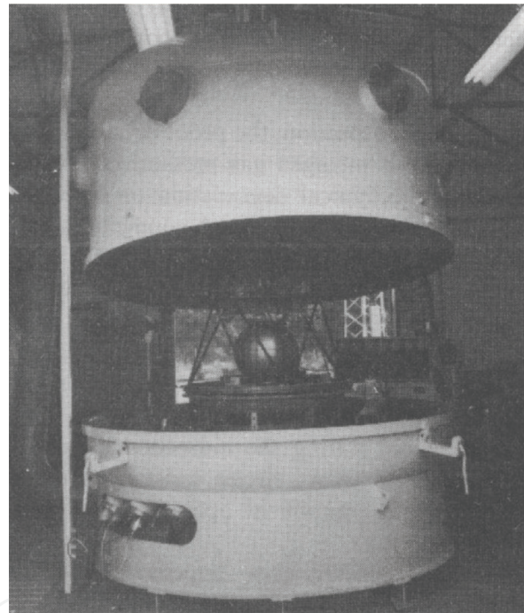
Figure 7. Entire system EM testing vacuum chamber [1].
