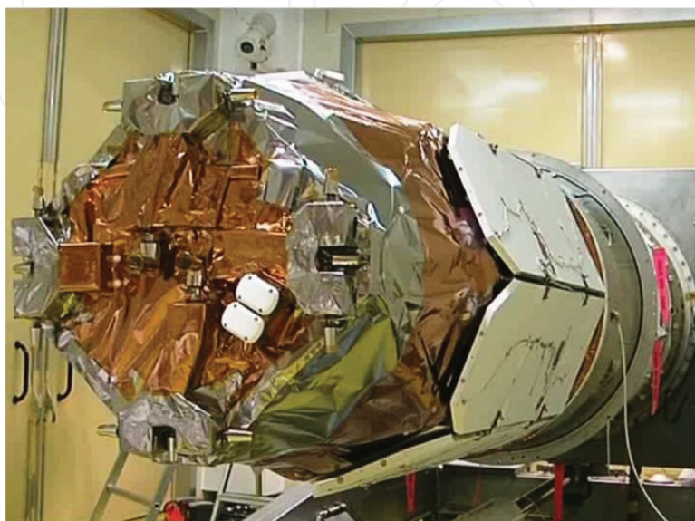
Figure 1. Offek satellite top plate with monopropellant hydrazine thrusters [2].
