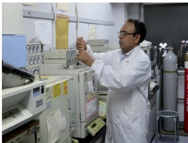
Figure 4. Injecting air samples into GC for determination of CH 4 and N 2 O concentrations.
