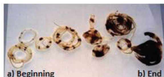
Figure 2. Evolution of hot spot during MW drying of onion slices [10].
