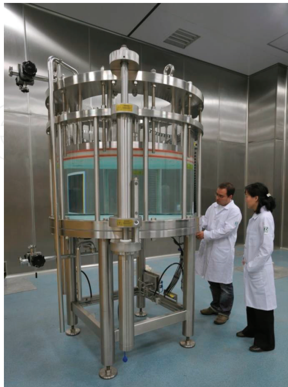
Figure 6. One of the larger chromatography columns of plasma fractionation plant (Instituto Butantan Foundation).
